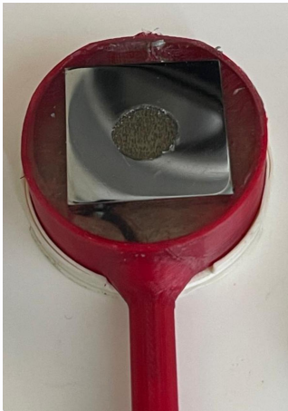
Figure 7: Embedded sample after test, with corroded region
