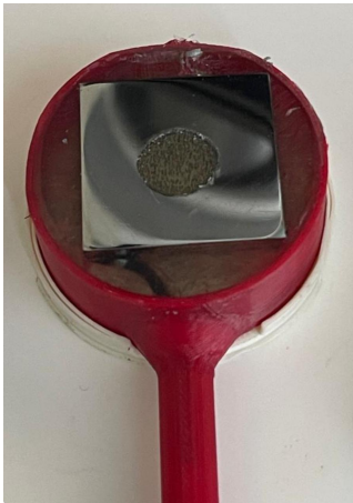
Figure 7: Embedded sample after test, with corroded region
