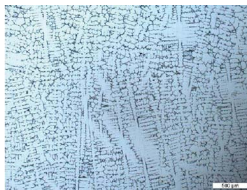
Stellite 31 cast microstructure
