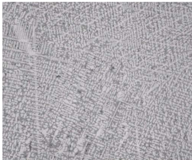
Optical Micrograph of a Stellite 12 PTA Deposit at 500X.
